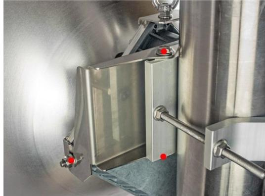
**8** Additionally, tighten the following screws marked with red dots on the left side view of the mounting bracket: left side screw on INTEGRAL-W FODU and two hex flange bolts between both mounting bracket clamps for housing and pipe with torsion 20..25 N-m.
