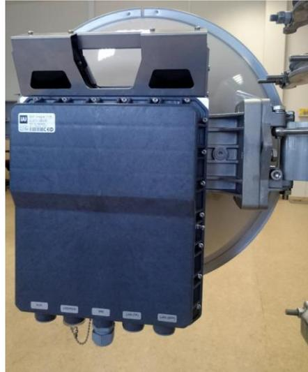
6 Final view of assembled INTEGRAL-WS 6-13GHz\* 1+0 setup.
