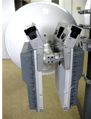
**6** Final view of assembled INTEGRAL-WS 6-13GHz\* 2+0 setup.
