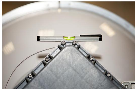
6 Verify polarization accuracy with a level, by placing it on the top edge of the INTEGRAL-WS housing
