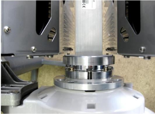
**5** Tighten all 4 INTEGRAL fixation clamps on both FODUs. When properly attached there's a gap between FODUs, OMT and antenna.
