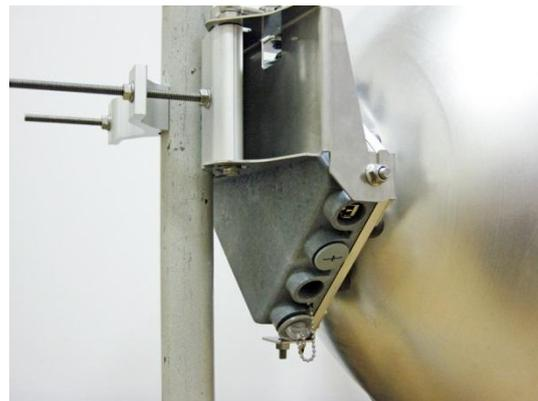
12 View of the assembled bracket on the mast pole with INTEGRAL-W FODU attached and secured.
