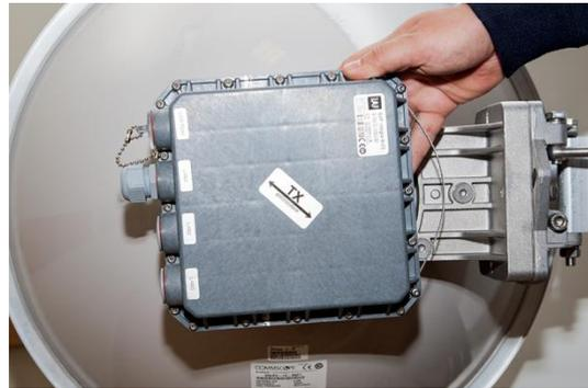
4 Rotate INTEGRAL-WS to match the required polarization.
