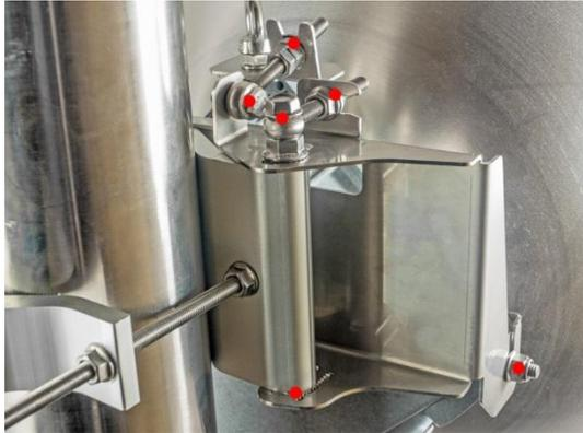
**7** When alignment is finished tighten screws marked with red dots on the right side view of the mounting bracket: hex flange nuts and bolts of azimuth and elevation eye screws, right side screw on INTEGRAL-W FODU and hex flange bolt on azimuth angle indicator with torsion 20..25 N-m.
