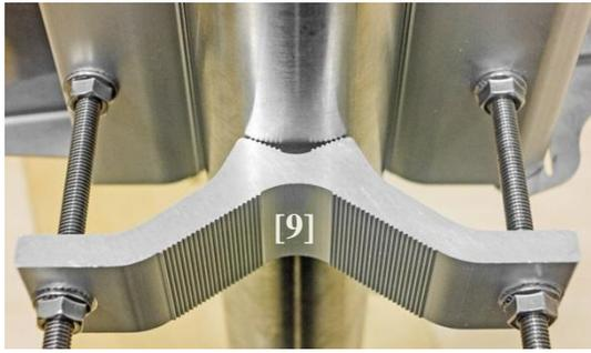
7 Hex flange nuts should be evenly aligned on threaded bolts so that mounting bracket clamp [9] is tightly attached to the pipe. Tighten hex flange nuts with torsion not exceeding 20 N·m.
