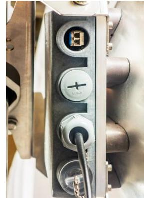
2 Unscrew the cap of the SFP port (LAN2 or LAN3) that will be used and install an SFP module.
