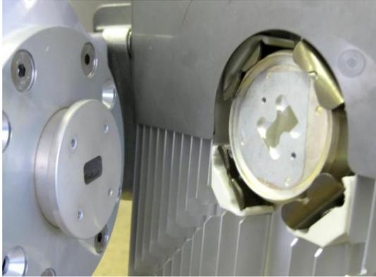
1 INTEGRAL-WS 6-13GHz\* FODU features twisted polarization flange and resulting signal polarization is determined by Interface on antenna/OMT. To change signal polarization, please rotate only the antenna interface, as radio always remains in vertical position.
