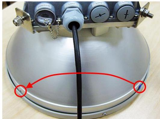
5 When polarization is changed, make sure that the drain-hole cap located at grounding flange nut is removed and inserted into the previous drain hole.
