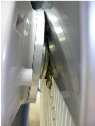
3 Put INTEGRAL-WS on antenna adapter flange by hooking half-turn loosened clamp at the top and leaving the completely loosened clamp at the bottom. Make sure O-ring is in place and the adapter flange fits into the INTEGRAL-WS transition flange socket.
