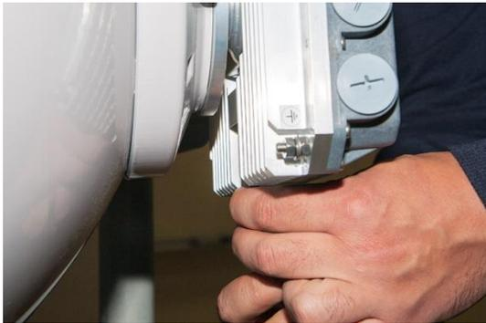
3 Secure the interconnection by tightening the bottom clamp (not fully). Make sure rotation of the INTEGRAL-WS is still possible.
