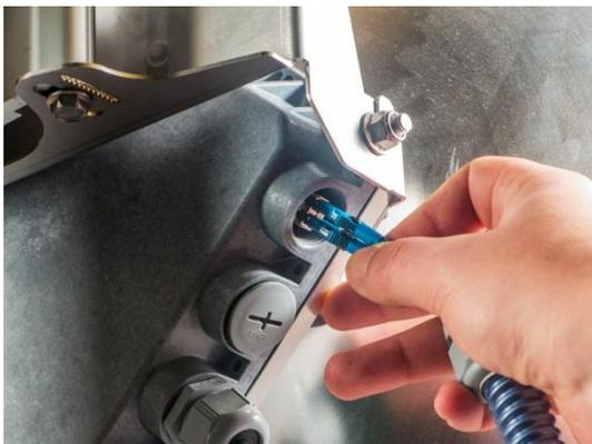
5 Connect LC connector to SFP module.
