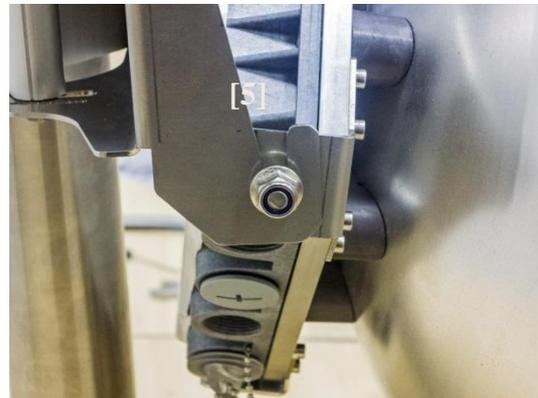
10 Attach INTEGRAL-W FODU with the antenna to the mounting bracket so that side screws fit into grooves of the housing clamp [5].
