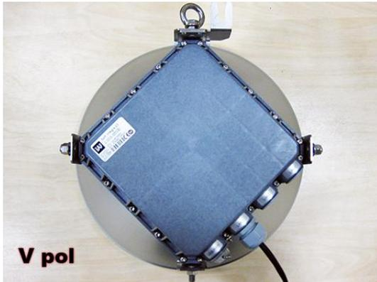
1 Remove INTEGRA-W FODU with an antenna from mounting bracket. Default polarization is vertical.
