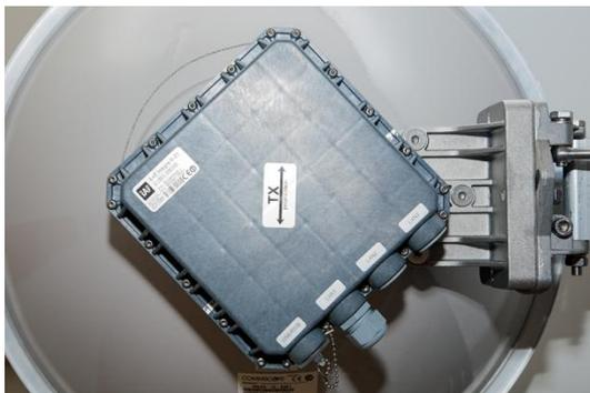
5 The sticker on the back lid indicates the polarization of the INTEGRAL-WS. Adjust polarization so that the interface ports are located at the lower side of the INTEGRAL-WS.
